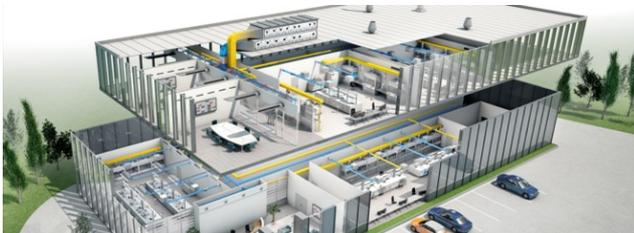
X-CUBE air handling units handle volume flow rates of up to 100,000 m<sup>3</sup>/h (28 m<sup>3</sup>/s) for the ventilation and air conditioning of rooms – including filtration, heating, cooling, heat recovery, and humidifying and dehumidifying
