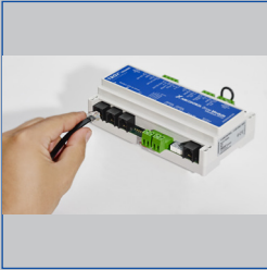
Zone module with plug-in connections for plug and play
