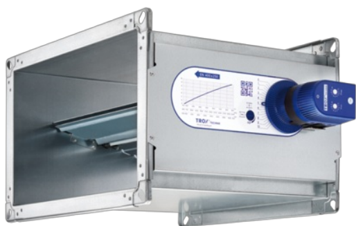
CAV controller of Type EN for higher volume flow rates 40 – 3.360 l/s 144 – 12.096 m 3 /h B: 200 – 600, H: 100 – 600 mm \Delta p : 50 – 1.000 Pa Casing air leakage to EN 1751, class C
