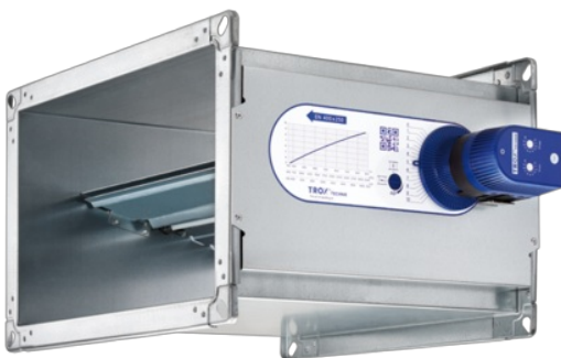
CAV controller of Type EN for higher volume flow rates 40 – 3.360 l/s 144 – 12.096 m³/h B: 200 – 600, H: 100 – 600 mm \Delta p : 50 – 1.000 Pa Casing air leakage to EN 1751, class C
