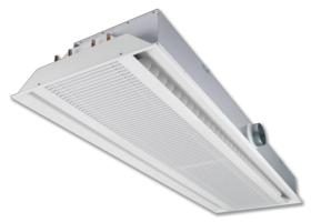
Active chilled beam DID632 Primary air: 6 - 85 l/s 22 - 306 m³/h L: 900 - 3,000 mm B: 593, 598, 618 und 623 mm H: 210 mm
