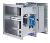
Fire dampers must close at a certain temperature or when smoke is detected. They effectively close off adjacent fire compartments and prevent the spread of fire and smoke.
