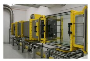
A test rig for testing coarse and fine dust filters according to EN779 is the fundamental component of our filter laboratory.
